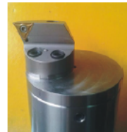
80mm bar with CH-5 head using TCMT 1604 insert
