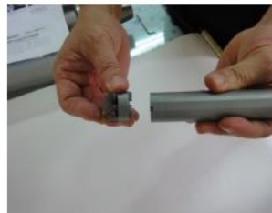
Remove screws & align cutting head to bar
