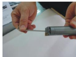
Check head alignment is correct, insert screws & tighten
