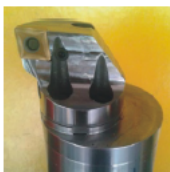
50mm bar with CH-5 head using CNMG 1204 insert
